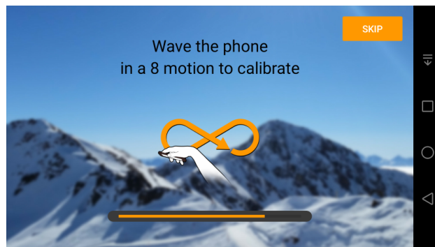
Figure 3.8: Orientation Sensors Calibration: how to move the device to help the sensor calibration.
